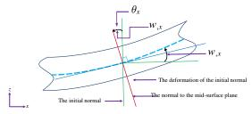
• Independent discretization of the displacement and the rotation field:
