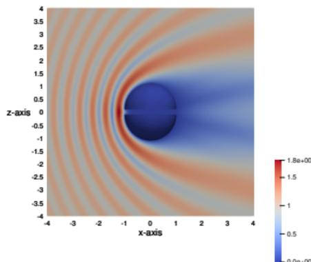
Figure: Acoustic scattering of a plane wave by half-spheres in 3D ( $\delta = 0.1$ ).
