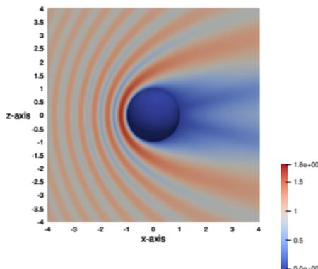
Figure: Acoustic scattering of a plane wave by half-spheres in 3D ( $\delta = 0$ ).
