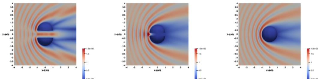
Figure: Acoustic scattering of a plane wave by half-spheres in 3D.
